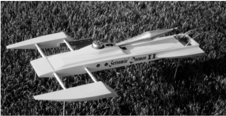
Fig. 2: The Roadrunner outrigger hydroplane.
